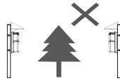
② There are obstacles such as trees between the transmitter and receiver.
