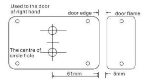
The weight of observation door and the implents of closing door (if being provided with the implements of closing door) cooperate whether to desire. When closing the door and if discovering the largenoise or not to lock you may serowthe six angle nut with 12# spanner or pincers (as following map) and adjust the loading spring repeatedly until loose and tight balance as you open or close the door.
