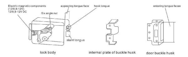
When the hook tongue and the slant tongue are installed on the contray the internal unlock can be become external unlock, the method of installation is the same. After the locks are installed well the doors are closed namely the locks are done steady automatically.
