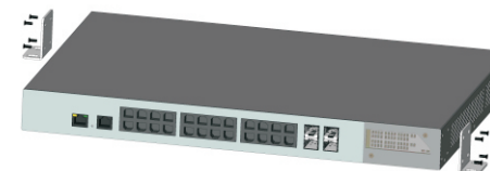
Figure 2-3 Hangers installation diagram
