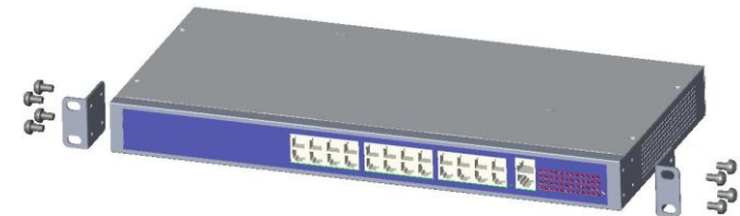
Figure 2-1 Install hangers diagram
