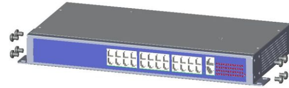
Figure 2-3 Hangers installation diagram
