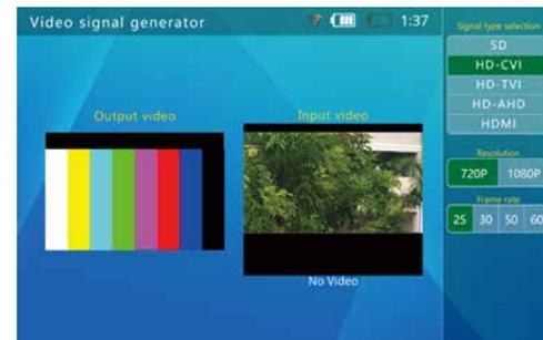
“System select”: Test image format, which supports the format selection of SD (PAL and NTSC), HD-CVI, HD-TVI, AHD, HDMI.
