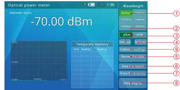
After Connecting the optical fiber to be tested into Fiber IN port of the tester, the tester will display measured laser power value.
