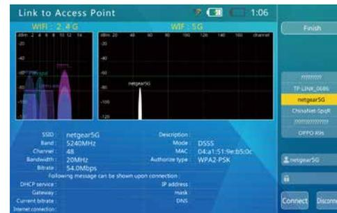
Select the name of wireless network that needs to be connected to, and then enter the password. At this time, the designated WIFI network will be connected to just by clicking “Connecting to WIFI”.
