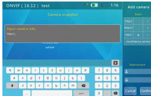
To manually add a camera, the user needs to know both IP address and ONVIF service path of the camera.
