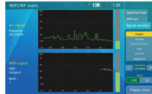
Click / select the hotspot in the right WIFI list, and then the “frequency” below will jump to the central frequency point of this hotspot channel; after that, start detecting the signal intensity at this frequency point. (as shown in the following figure)
