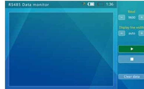
Click the button of “+ / -”, below “Baud rate”, and then set the baud rate, so as to make it be in line[fit match] with that of the measured RS485 bus. When the tester receives some data, these data will be displayed on the screen. Press it match to pause / resume receiving the data.
