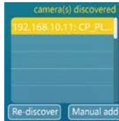
**!** Attention: When part of cameras cannot respond/appear on the "Camera list" due to they are located in different network segments, the user shall first return to Step 1, and then modify the IP of this device, so as to make it be in the same network segment of the camera (Please note that the IP can't conflict with other devices in the network after modification.); after that, enter Step 2, and attempt to discover the camera.
