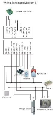
Diagram A instructions is electricity lock, using a special power supply access of the connection mode; Diagram B instructions is electricity lock and fingerprint access to share a power supply. Special attention: to protect the power supply, locks needed to mount a diode in the positive and negative ends, and the white side marked on the diode connects to the electric lock positive.
